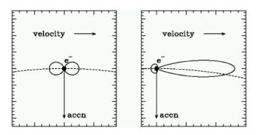
*Figure 1: Electron moving at non-relativistic (left) and relativistic (right) speeds*
