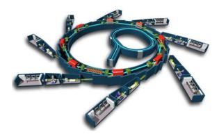
Figure 2: An image showing a synchrotron facility with the booster ring in the middle and the storage ring on the outside. The straight section connecting to the booster ring is the LINAC.
